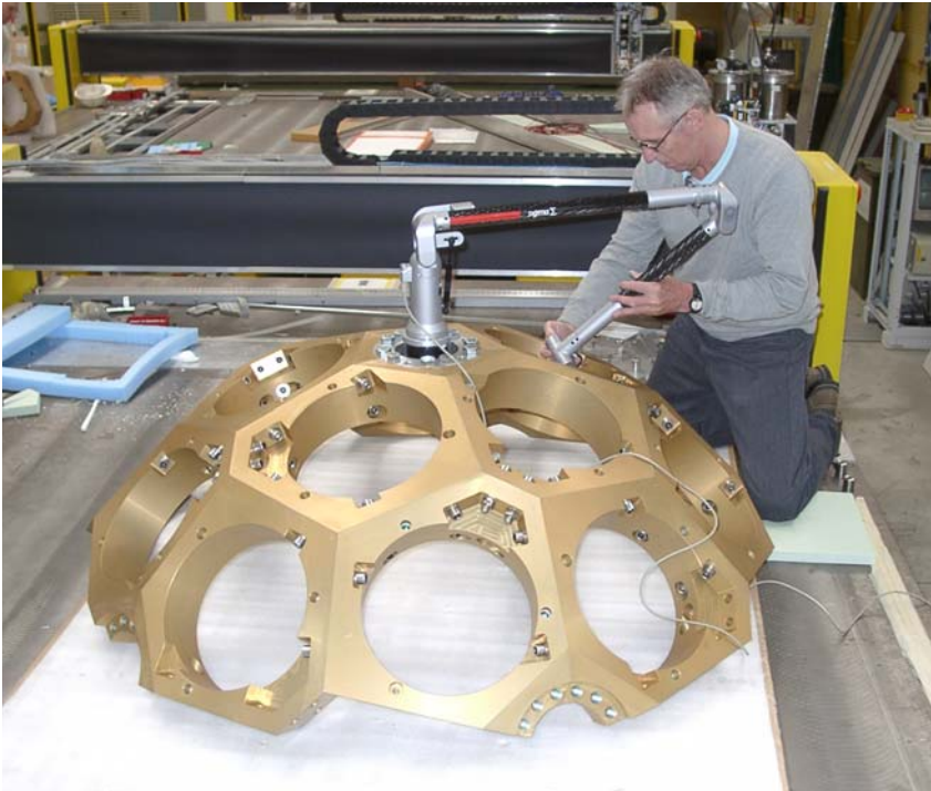
Flange Assembly measured initially with Romer Arm, and finally with Faro Laser Tracker.
