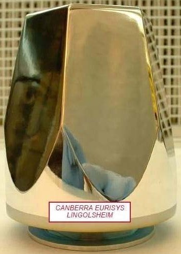
First AGATA triple cluster detector IKP Cologne, H.-G. Thomas CTT Montabaur
